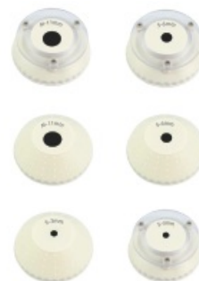
BGD 552/2 supports 6 measurement apertures for different sample sizes
