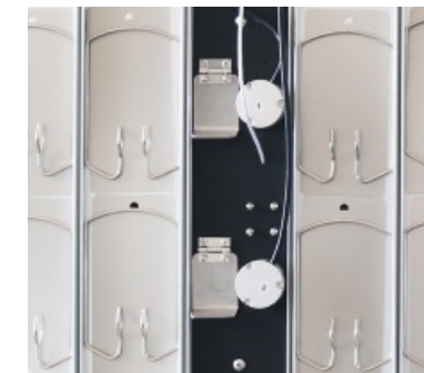
Four sensors monitor UV irradiance
