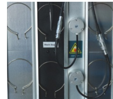
Four sensors monitor BUV irradiance
