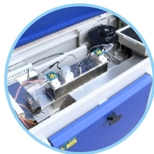
Flip design is convenient for lamp installation and maintenance
