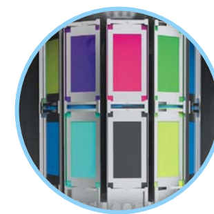
Rotating-drum design of sample holder
